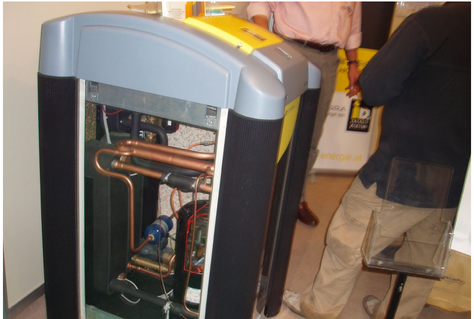
A geothermal heat pump has three components. Antifreeze runs through plastic pipes in the ground (not shown) to collect or deposit heat. Refrigerant runs in copper pipes to pull that heat out of the antifreeze. An air handler (not shown) then heats the premises through ducting. Geothermal heat pumps to baseboard are possible, too, although at time of writing less frequently commercially available. CC BY-SA 4-0 Tzeferis Petros.
