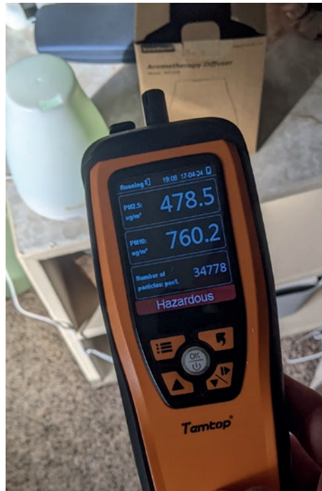
The air quality monitor doesn't lie: Not only was this fragrance diffuser setting off the smoke alarm, but it was also creating hazardous air quality conditions in the home. (License: CC by-sa MassLandlords Quattrochi)
