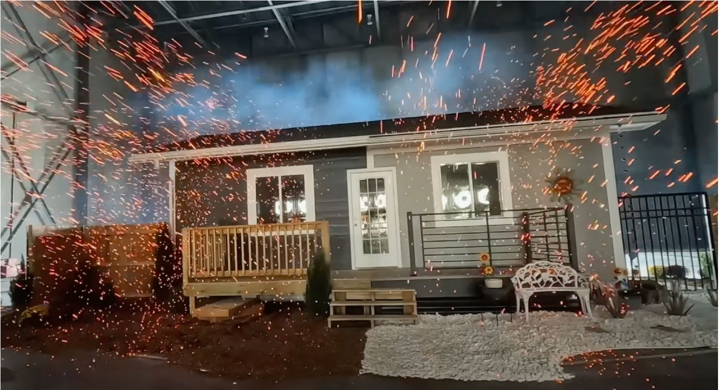
This Insurance Institute for Business and Home Safety lab allows scientists to do a side-by-side comparison of how structures fare in wildfire conditions. The left side of the house has not been hardened, the right side of the home has. (Image: Fair Use, PBS Terra “The Real Story of the LA Fires”)
